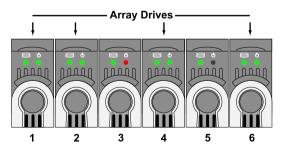
When the rebuild is complete, the spare drive has replaced the failed drive. In this example, failed drive 3 was replaced by spare drive 6. The disk array now consists of physical drives 1, 2, 4, and 6.
